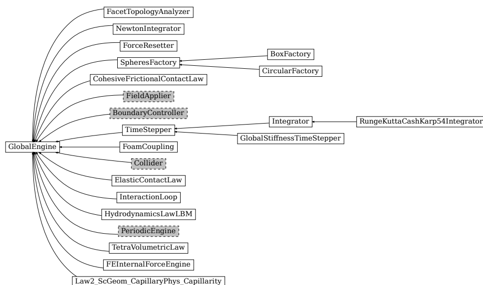
Fig. 25: Inheritance graph of GlobalEngine, gray dashed classes are discussed in their own sections: FieldApplier , BoundaryController , Collider , PeriodicEngine . See also: BoxFactory , CircularFactory , CohesiveFrictionalContactLaw , ElasticContactLaw , FEInternalForceEngine , FacetTopologyAnalyzer , FoamCoupling , ForceResetter , GlobalStiffnessTimeStepper , HydrodynamicsLawLBM , Integrator , InteractionLoop , Law2_ScGeom_CapillaryPhys_Capillarity , NewtonIntegrator , RungeKuttaCashKarp54Integrator , SpheresFactory , TetraVolumetricLaw , TimeStepper .
